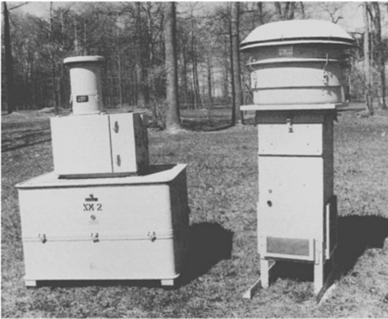
XM2/XM19 Biological Detection and Warning System. Each system stands about six feet tall. Courtesy of the U.S. Army
