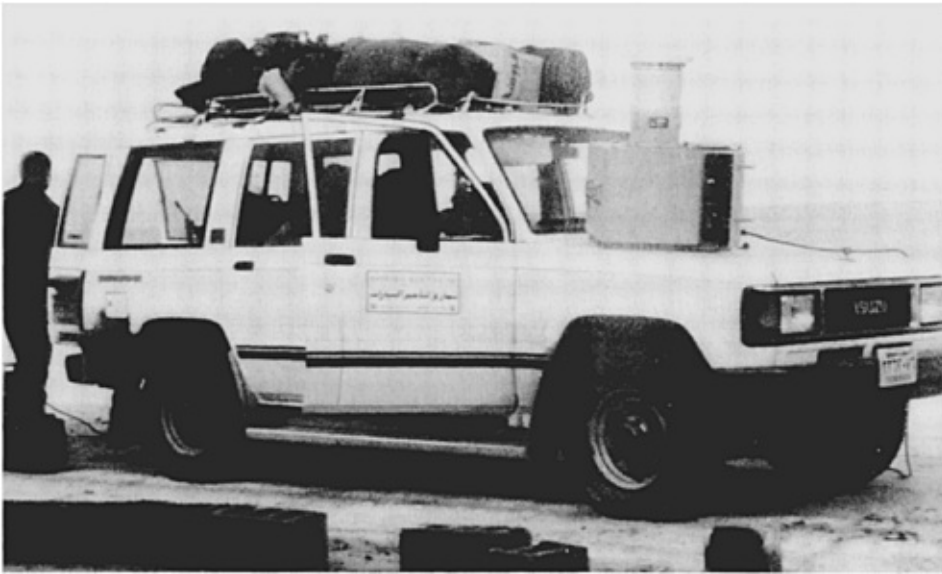
The Army's interim biological agent reconnaissance vehicle for the Gulf War was a leased Isuzu civilian truck with an XM2 Biological Sampler strapped to its hood. Courtesy of the U.S. Army
